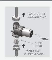
(EN) Note: Make sure the filter is located between the solenoid housing and the water inlet.
